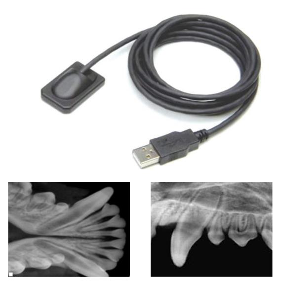
MasterDent is a CMOS area image sensor developed for High Quality X-ray imaging. The image sensor has 2.1 mega pixels (1300x1700) with a pixel size of 20x20 µm and a monitoring photodiode for monitoring and detecting X-ray radiation. FOP (fiber optic plate) used at the input window ensures high image quality and long sensor life. This product is dust and water proof.
